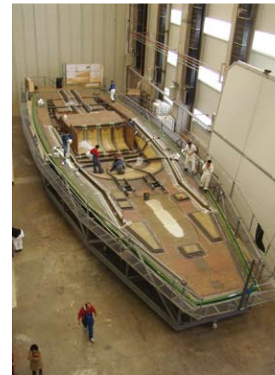
Preparing the 125 Flybridge deck moulding. Workers carefully lay the laminates of e-glass CSM and e-glass 0/90 biaxial and quadaxial that will sandwich a 25mm 150kg/m 3 balsa core
